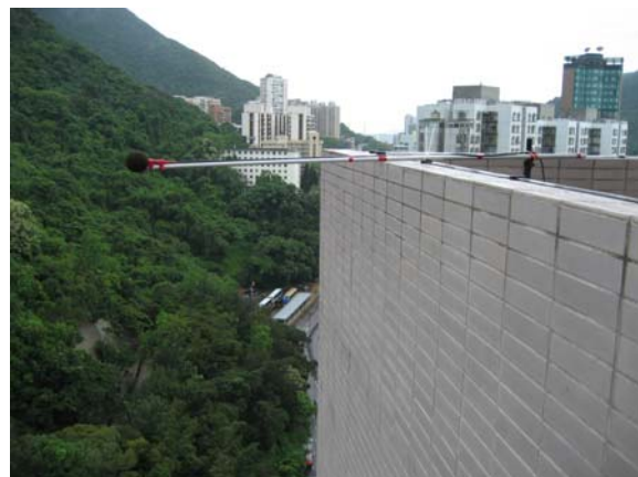
Baseline Noise Monitoring Station (NM2)
