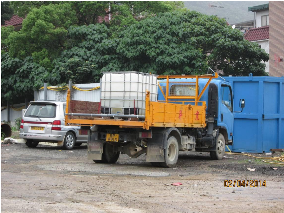
Fig.4 –Water spraying was provided by frontline staff for dust suppression.
