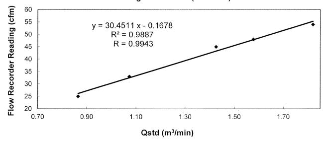
Acceptance Criteria : Correlation coefficient (r) of the calibration curve greater than 0.990 after a 5-point calibration
