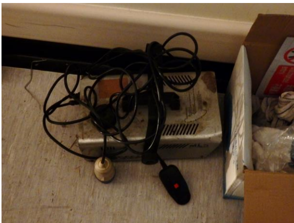
Figure 3.28 Smoke generator used for the smoke test at 5/F Incinerator Room
