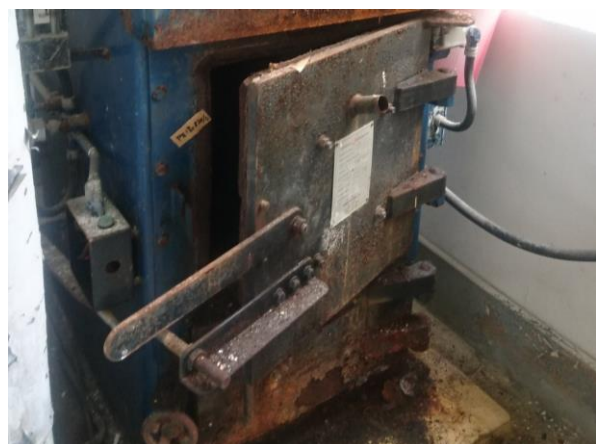
Figure 3.2 The incineration chamber door (top) and the bottom ash collection door (bottom) of the incinerator
