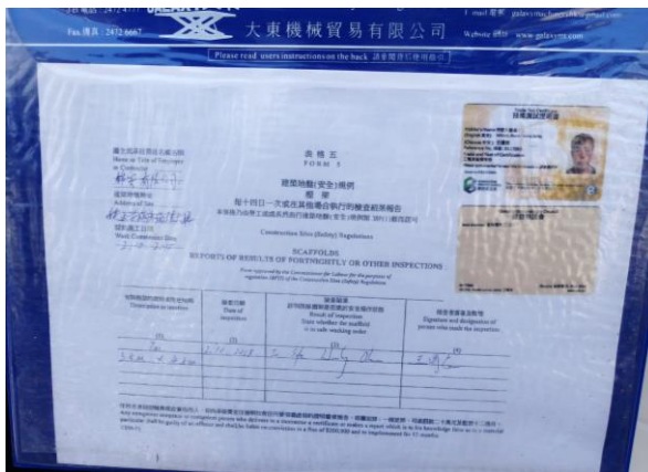
Figure 3.15 Inspection record for the scaffold
