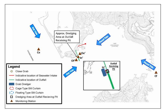
Figure 5.1 – Monitoring Stations of Silt Curtain Efficiency Testing
