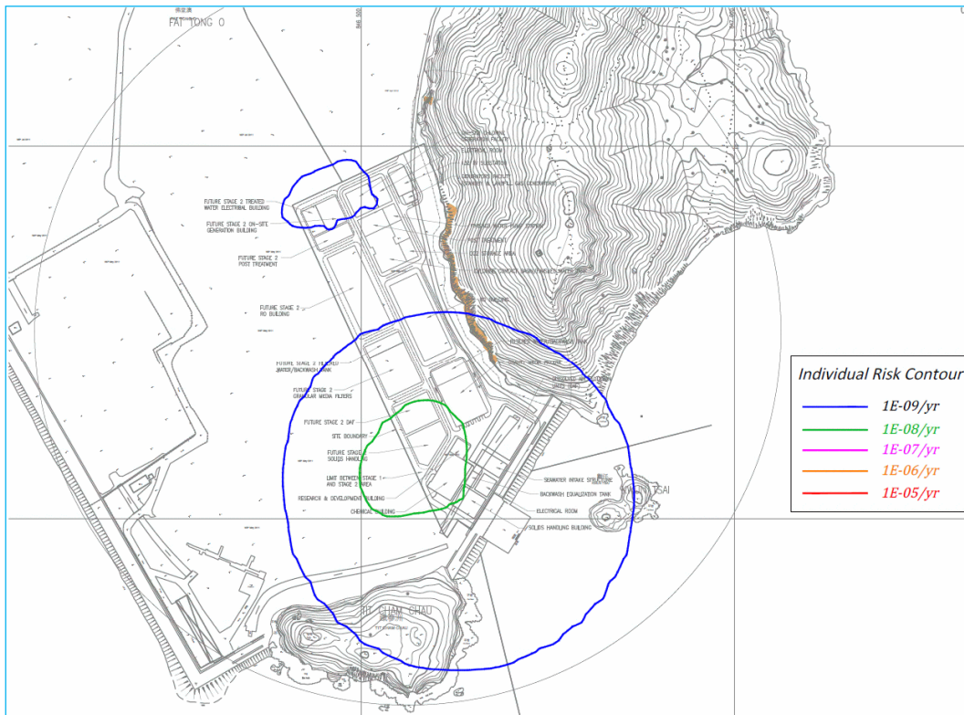
Figure 11.14 Individual Risk Contours for Sodium Bisulphite Assessment
