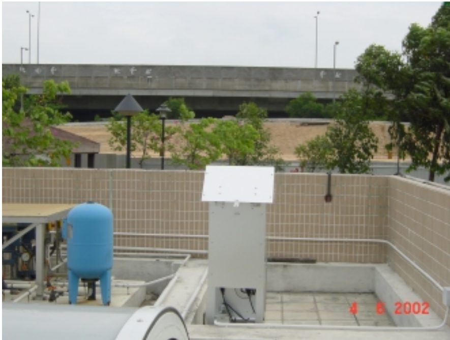
Air Quality (TSP) Monitoring Station at Lai Chi Kok Park of Mei Foo Sun Chuen
