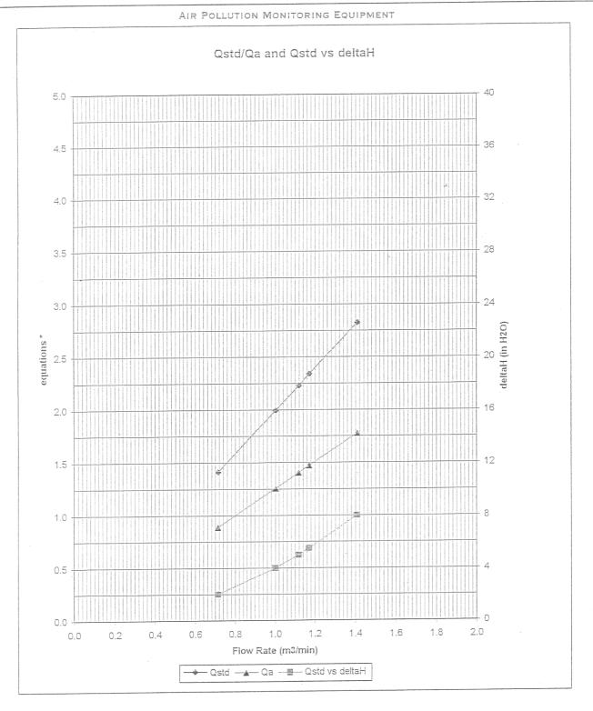
\* y-axis equations: Qstd series:  $\sqrt{\Delta H \left(\frac{Pa}{Pstd}\right) \left(\frac{Tstd}{Ta}\right)}$   $\sqrt{\left(\Delta H \left(Ta / Pa\right)\right)}$
