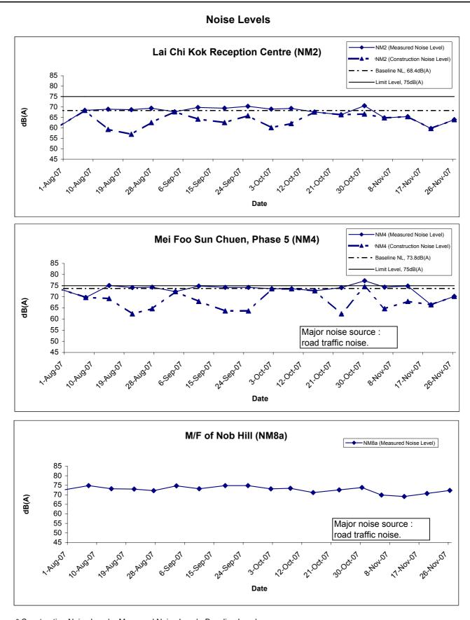
\* Construction Noise Level = Measured Noise Level - Baseline Level (If the measured noise level is lower than the baseline level, the construction noise level will be taken as the measured one)
