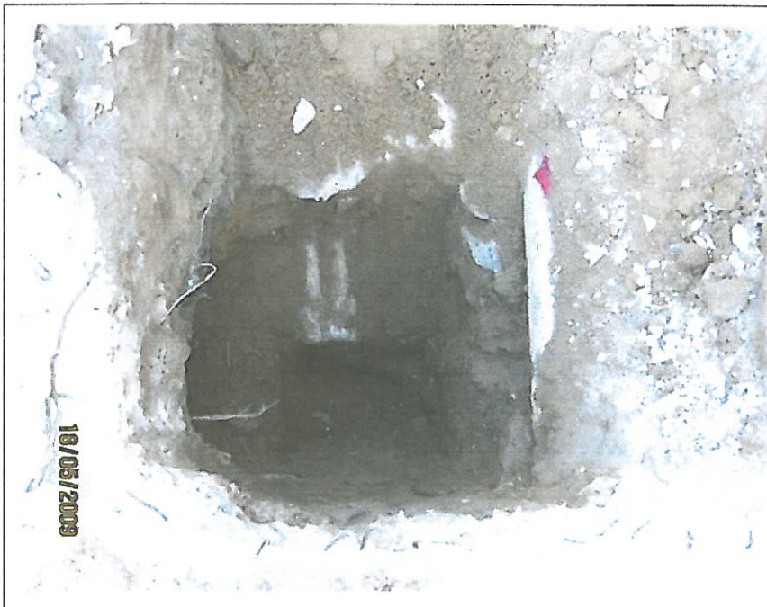
Top view of sampling locations at trial pit no. GFSA-05 below 0.5m and 1.5m BBC
