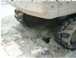
Oil leakage was observed. The Contractor should provide repairing and avoid further leakage for water or soil contamination.
