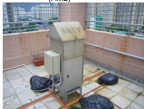
Photo 2.2 HVS installed at Tung Wah Group of Hospitals Tai Tung Pui Social Service Building (AM2)
