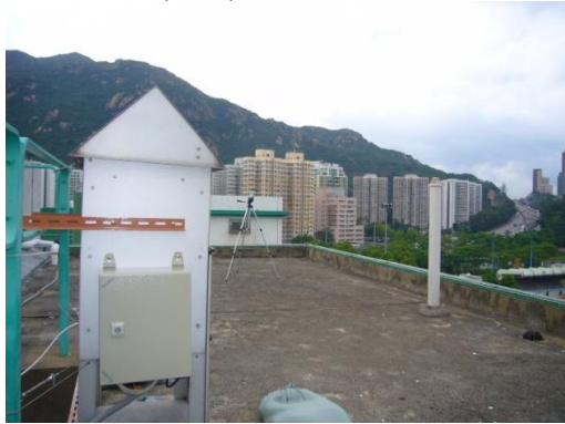
Photo 2.5 HVS installed at Tuen Mun Town Hall (AM5)
