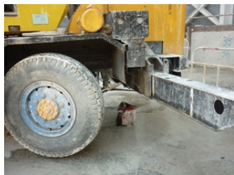
Photo 2: A leaking oil hydraulic excavator was observed
