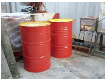
Photo 7: Chemical drums without drip tray
