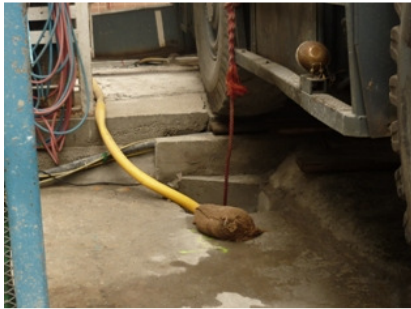
Photo 3 Trashes were found in drip tray under the air compressor
