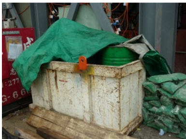
Photo 1 A chemical drum without labels was found
