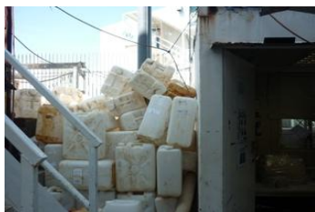
Photo 3 Chemical was found without drip tray on the access and near the noise enclosure
