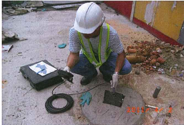
Photo 31 - Site B2 Temperature, Electrical Conductivity and pH Value Measurement at B-27
