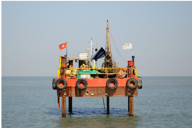
Vessel Particular for Marine GI Work
