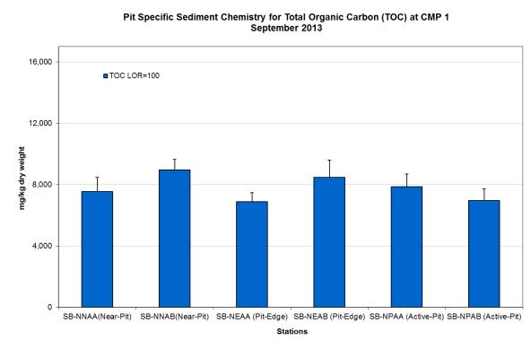
Figure 7: Concentration of Total Organic Carbon (mg/kg dry weight; mean +SD) in sediment samples collected from Pit Specific Sediment Chemistry Monitoring for CMP 1 in September 2013.
