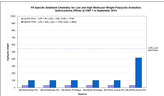
Figure 9: Concentration of Low and High Molecular Weight Polycyclic Aromatics Hydrocarbons (PAHs) ( $\mu$ g/kg; mean +SD) in sediment samples collected from Pit Specific Sediment Chemistry Monitoring for CMP 1 in September 2013.
