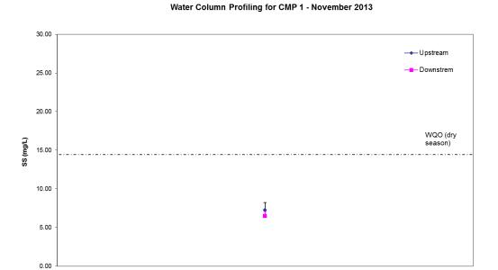
Figure 13: Suspended Solids (mean + SD) recorded during Water Column Profiling for disposal operations at CMP 1 in November 2013.
