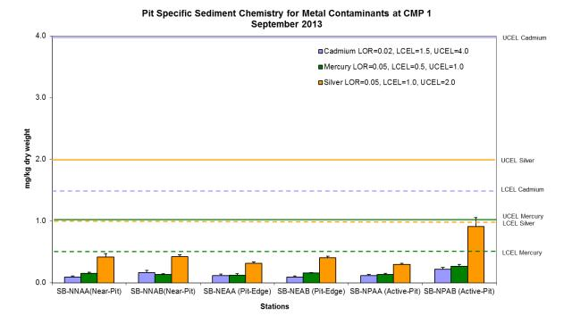
Figure 6: Concentration of Metals (Cd, Hg, Ag; mean +SD) in sediment samples collected from Pit Specific Sediment Chemistry Monitoring for CMP 1 in September 2013.
