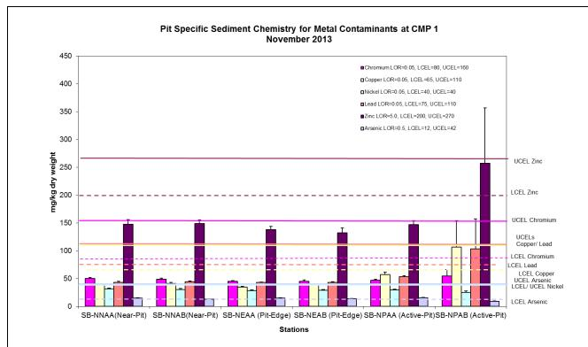
Figure 24: Concentration of Metals (Cr, Cu, Ni, Pb, Zn, As; mean +SD) in sediment samples collected from *Pit Specific Sediment Chemistry Monitoring* for CMP 1 in November 2013.
