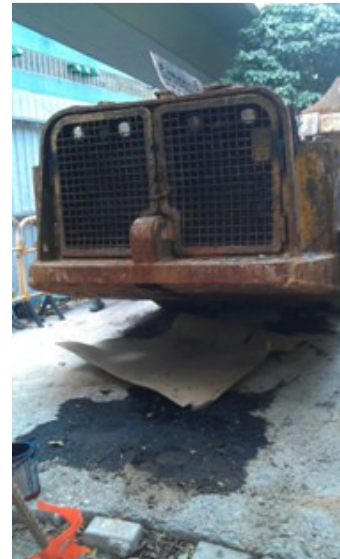
Photo 4 Oil leakage from a plant was found in the storage area.
