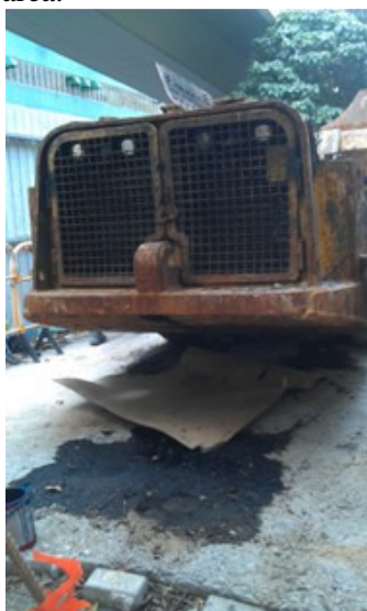
Photo 3 Oil leakage from a plant was found in the storage area.
