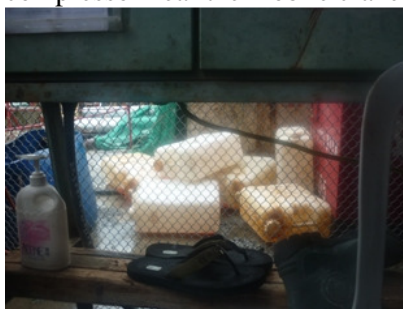
Photo 2 Some chemical drums were found without suitable labels and drip tray next to air compressor near the mobile crane
