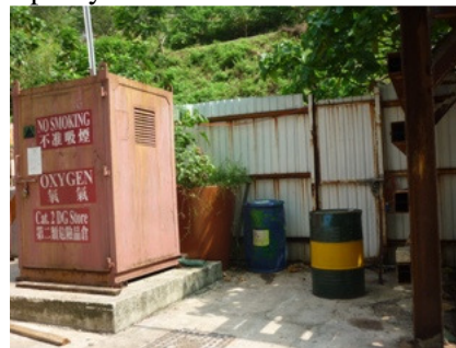
Photo 4 Some chemical barrels were found in the workshop without suitable labels and drip tray
