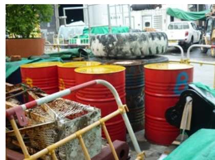
Photo 2 Oil barrels were found without drip trays
