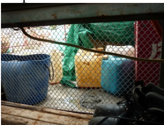
Photo 1 Some chemical drums were found without suitable labels and drip tray next to air compressor near the mobile crane.
