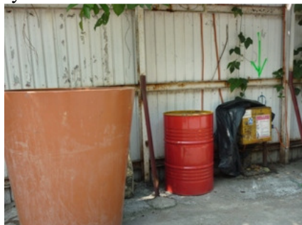
Photo 3 Some chemical barrels were found in the workshop without suitable labels and drip tray
