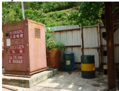
Photo 4 Some chemical barrels were found in workshop without suitable labels and drip tray
