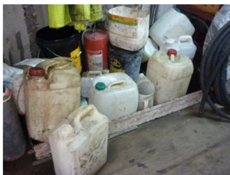
Photo 3 Chemicals without labels were found in plant container
