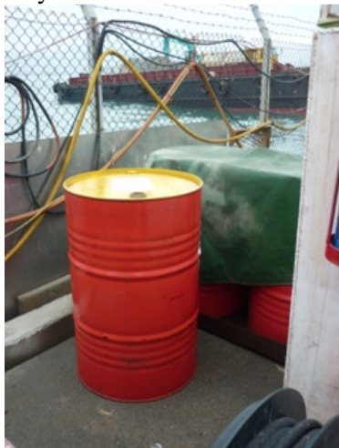
Photo 1 An unknown chemical drum without drip tray was found next to the fuel tank.
