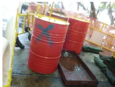
Photo 2 Some chemical barrels were found without drip tray next to chemical storage since last inspection
