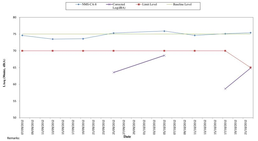
Examination was undertaking during the monitoring on 22th October 2012. The limit level is 65dB(A).
