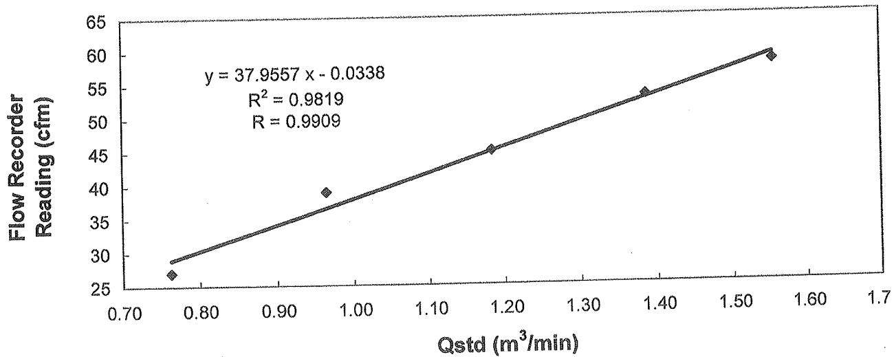
Acceptance Criteria : Correlation coefficient (r) of the calibration curve greater than 0.990 after a 5-point calibration
