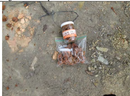
Photo 6: Soil Sample CW-04/2/1.5m bgl
