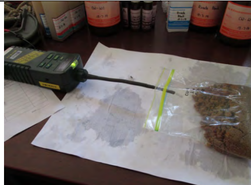
Photo 6: Photo-ionization Detector (PID) was used to measure headspace vapor concentration
