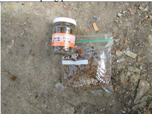
Photo 7: Soil Sample CW-03/2/1.5m bgl
