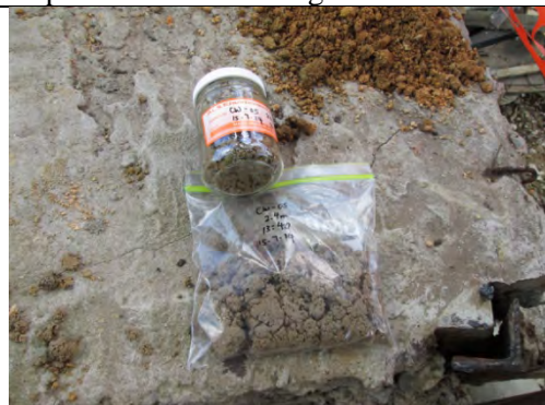
Photo 8: Soil Sample CW-05/3/2.4m bgl
