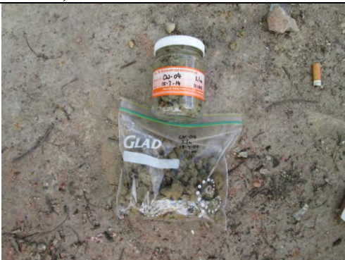
Photo 7: Soil Sample CW-04/3/3.1m bgl
