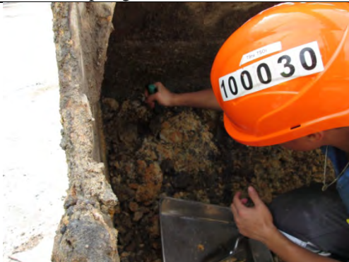
Photo 3: Soil sampling process at the bucket of excavator
