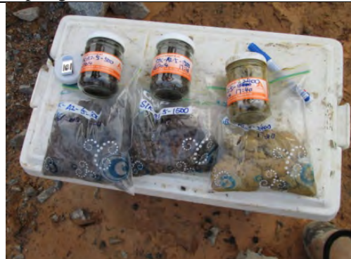
Photo 4: Soil Samples: STK-A2-5/1/0.5m bgl, STK-A2-5/2/1.5m bgl and STK-A2-5/3/2.4m bgl
