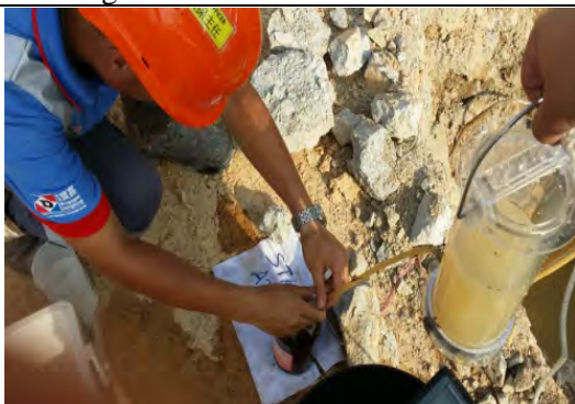
Photo 7: Groundwater sampling process
