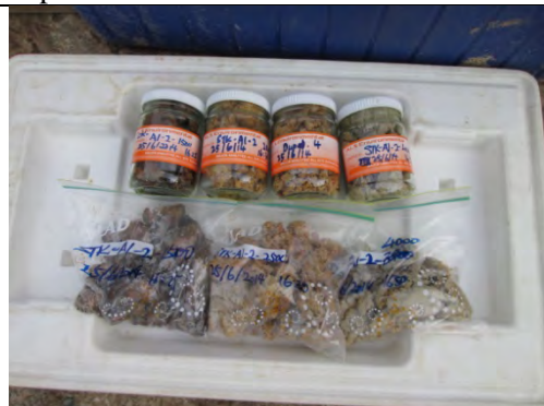
Photo 6: Soil Samples: STK-A1-2/1/1.5m bgl, STK-A1-2/2/2.5m bgl; STK-A1-2/3/4.0m bgl and Duplicate sample Dupl-4
