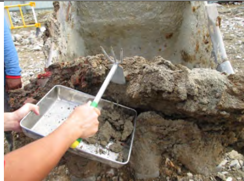
Photo 2: Soil sampling conducted at the bucket of excavator
