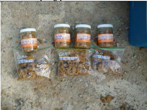
Photo 5: Soil Samples: STK-A2-2/1/1.0m bgl, STK-A2-2/2/2.0m bgl, STK-A2-2/3/3.1m bgl and Duplicate Sample
