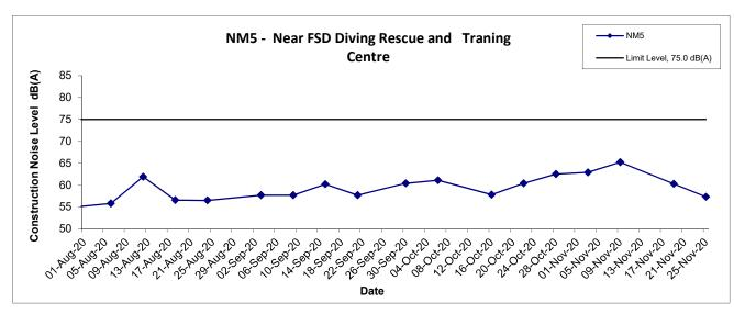
Contract No. DC/2009/10 Scale Project HATS 2A - Upgrading Works at SCISTW-N.T.S No. MA11007 Main Pumping Station, Sedimentation Tanks and Ancillary Date Appendix Graphical Presentation of Noise Monitoring Result Nov 20
