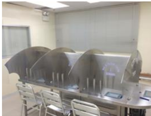
Figure 3: Olfactory Laboratory with Scentroid™ SS600 Olfactometer
