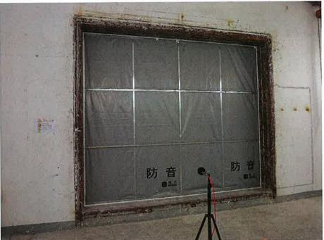
Set-up of Unit Under Test (Source room)
