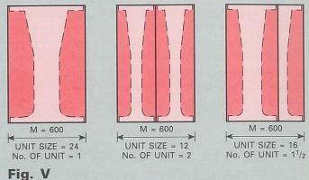
Each of the three configurations bears unique insertion loss and pressure drop performance. The final choice will rely on the actual noise control requirement and system layout.
