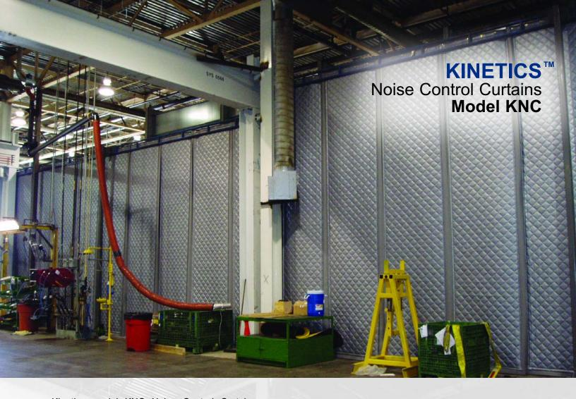
Kinetics model KNC Noise Control Curtains are modular, reinforced limp-mass and quilted fiberglass composites designed to block noise or to act as a movable barrier between noisy and quiet areas. Kinetics Noise Control Curtain Systems incorporate a self-supporting track which allows the curtain to open for access at virtually any point along the barrier or enclosure.
