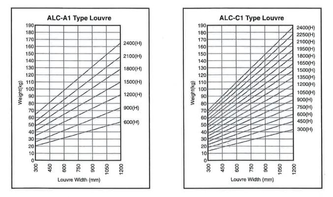
For ALC-A.5 and ALC-B2 Models, take the weight from the ALC-A1 Chart and Multiply by 0.5 and 2 respectively For ALC-C.5 and ALC-C2 Models, take the weight from the ALC-C1 Chart and Multiply by 0.5 and 2 respectively
