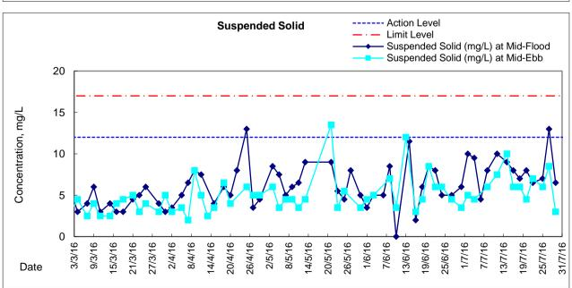
The construction work during the reporting period include, structural works for tunnel construction, roadworks, drainage works, seawall modification and removal of bulk head wall. The weather condition during the reporting period ranges from mostly sunny to rainy. The quarterly mean of suspended solids in this reporting quarter was found to be 6.5 mg/L which was lower than ambient mean of 7.5 mg/L according to the baseline monitoring data.
