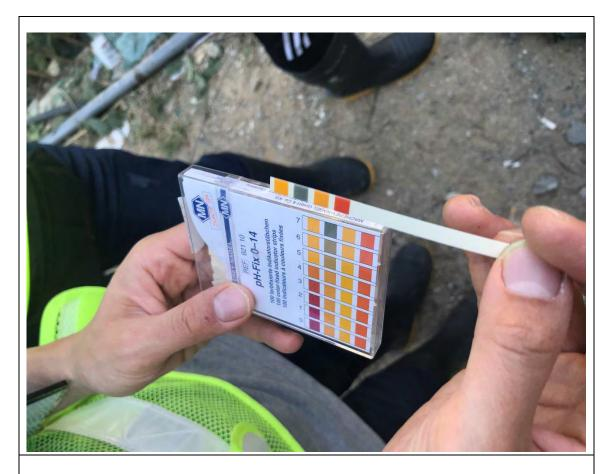
Water sample was collected at the stormwater terminal discharge point on 21 December 2018, and the pH tested with pH paper was approximate 7.
