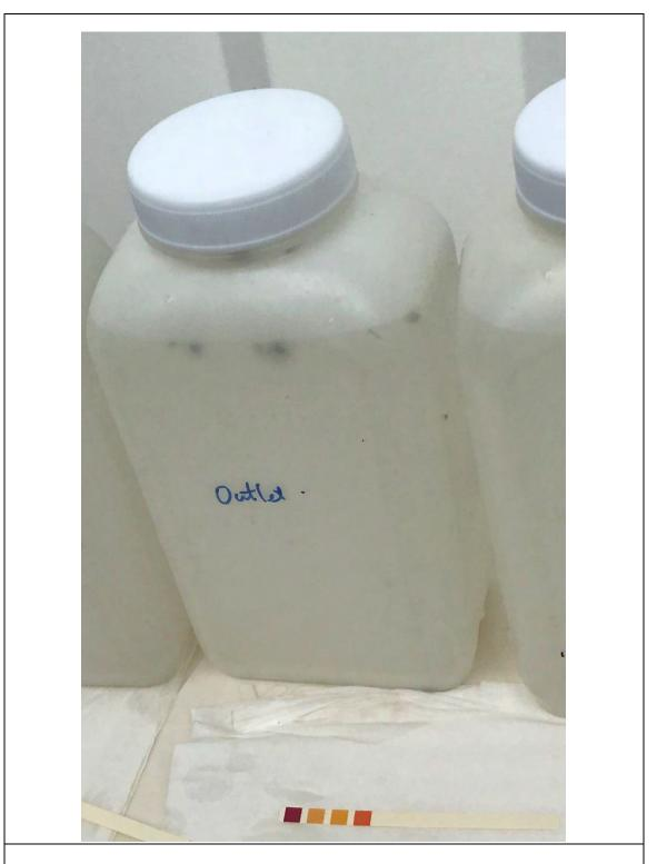
Water sample was collected at the stormwater terminal discharge point on 20 December 2018, and the pH tested with pH paper was approximate 1-2.
