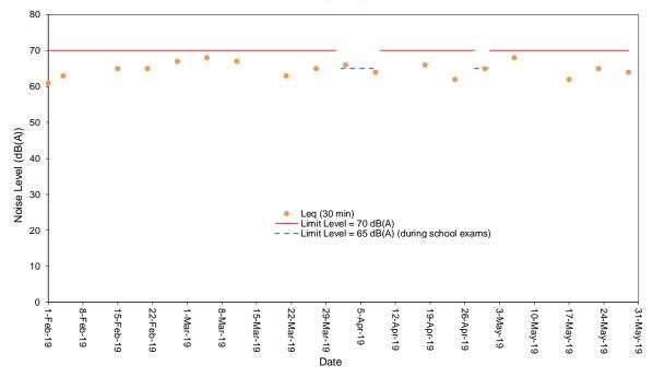
Remark: The measured noise level recorded at NMS3C on 2 April 2019 was 65.9 dB(A), which exceeded the noise Limit Level of 65 dB(A) during examination period at Ho Yu College but it was below the baseline level. Therefore, it is not considered as an exceedance. As such the Event and Action Plan was not triggered.
