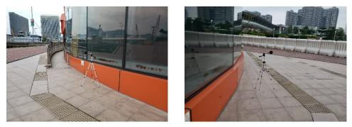
The station set-up of a façade measurement at station NM2A.
