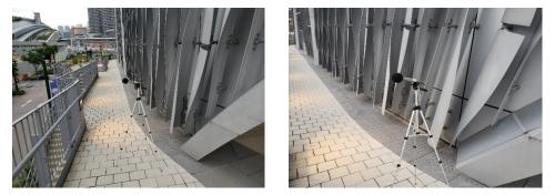
The station set-up of a façade measurement at station NM3A.
