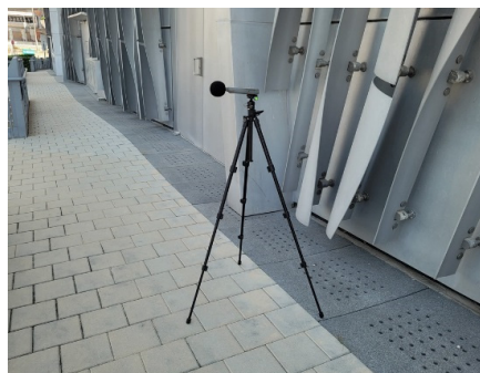
The station set-up of a façade measurement at station NM3A.
