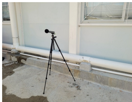
The station set-up of a façade measurement at station NM4A.
