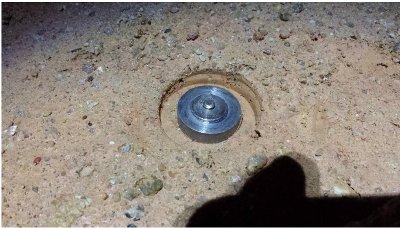
Spike for Setting Accelerometer on ground
