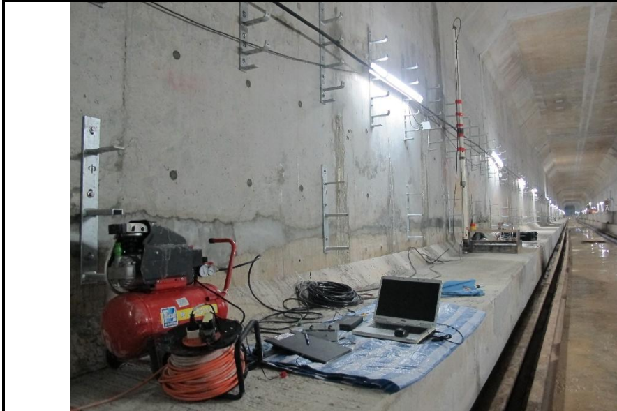
Hammer Impact Test in the Tunnel
