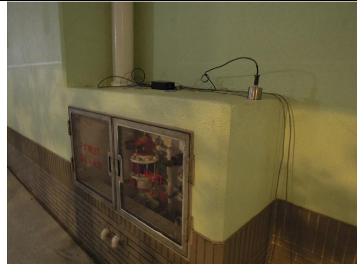
Point B (Accelerometer on Outdoor Building Structure)
