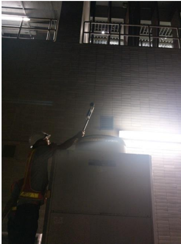
SWL Measurement for Outdoor Unit B
