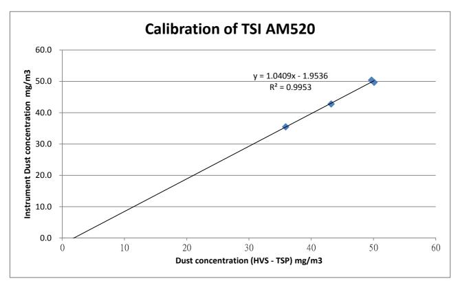
\*\*\* Filter paper being used in the calibration : 203475, 203476, 206020, 206603 Those filter papers are weighted by HOKLAS laboratory (ALS Technichem (HK) Pty Ltd.)
