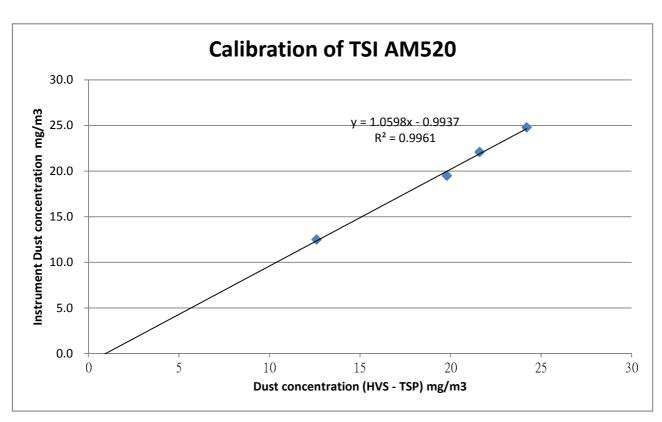
\*\*\* Filter paper being used in the calibration : 207858, 207859, 207860, 207861 Those filter papers are weighted by HOKLAS laboratory (ALS Technichem (HK) Pty Ltd.)
