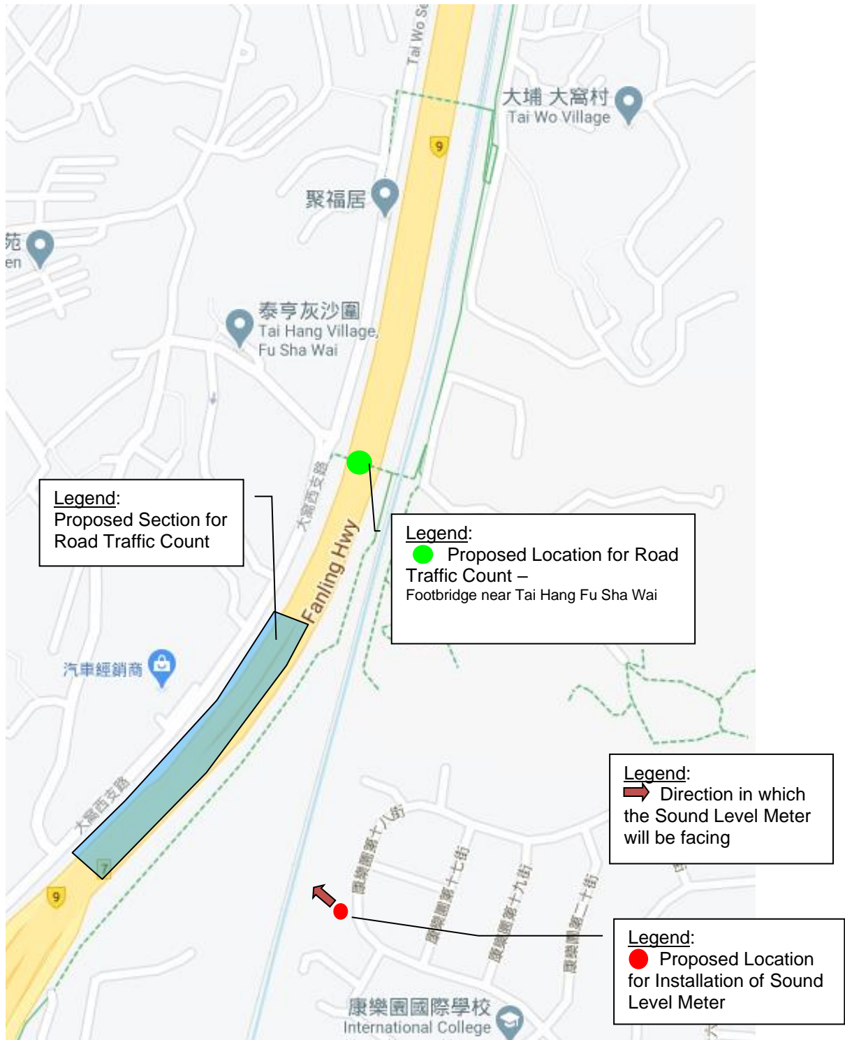
Figure 3 Proposed Road Traffic Count Map Location for Footbridge near Tai Hang Fu Sha Wai
