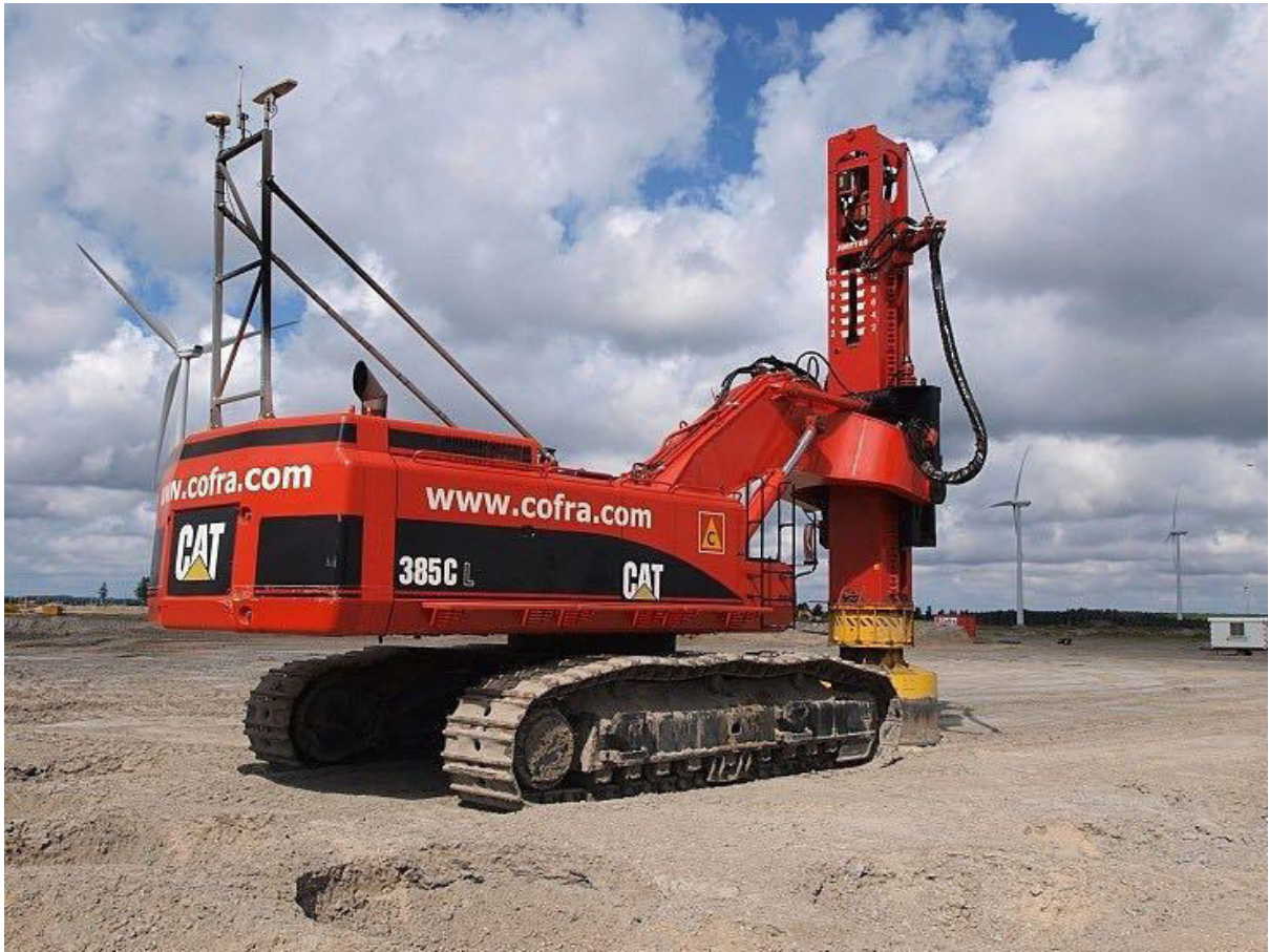
Band Drain Machine is modified by the excavator
