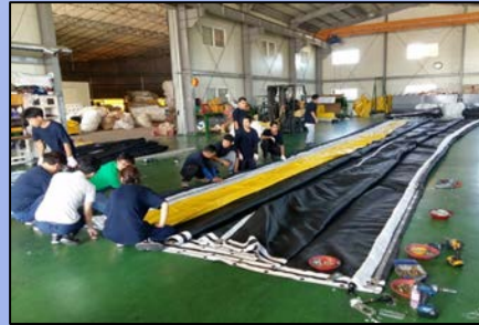
Fabrication of silt curtain
