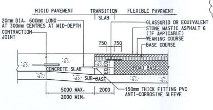
TRANSITION DETAILS BETWEEN RIGID PAVEMENT AND FLEXIBLE PAVEMENT N.T.S.
