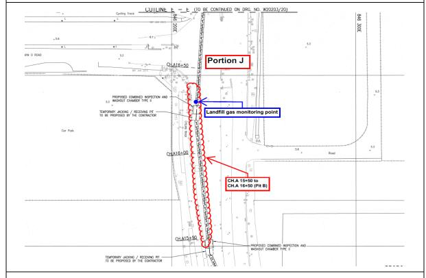
Figure 4.4 Monitoring Location – CH.A 15+50 ~16+50 (Jacking Pit B)
