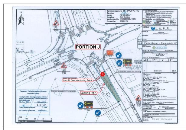
Figure 4.3 Monitoring Location – CH.A 13+50 ~ 14+00 (Pit A)
