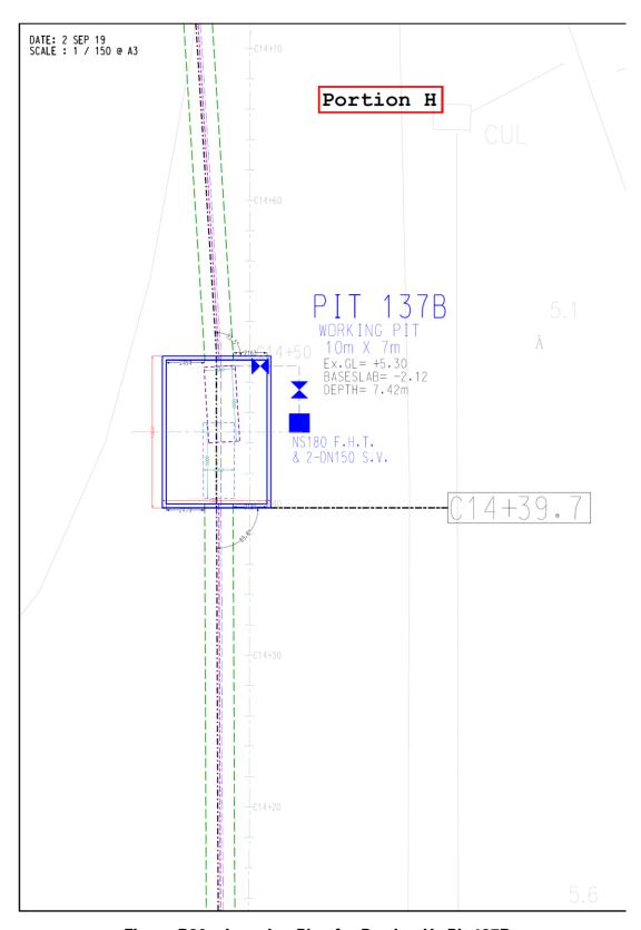
Figure B20a. Location Plan for Portion H- Pit 137B
