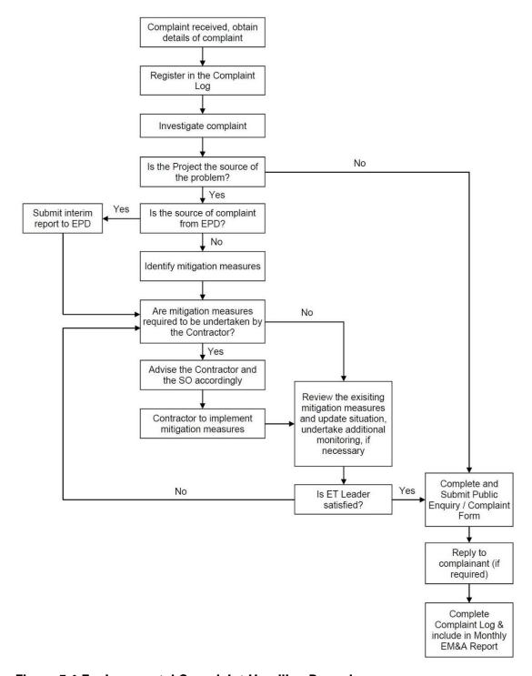
Figure 5.1 Environmental Complaint Handling Procedure
