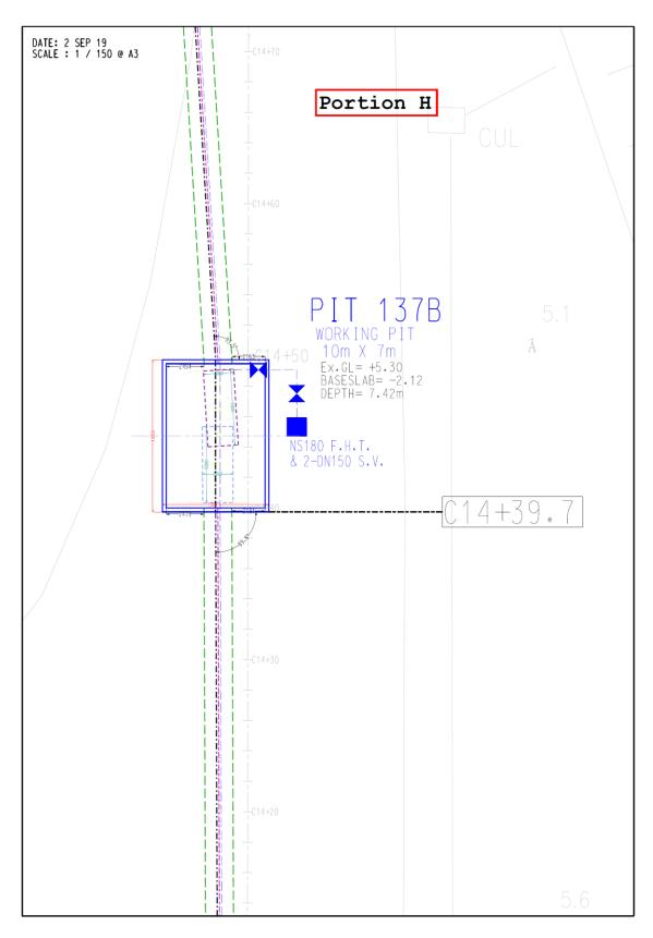
Figure B8. Location Plan for Portion H- Pit 137B
