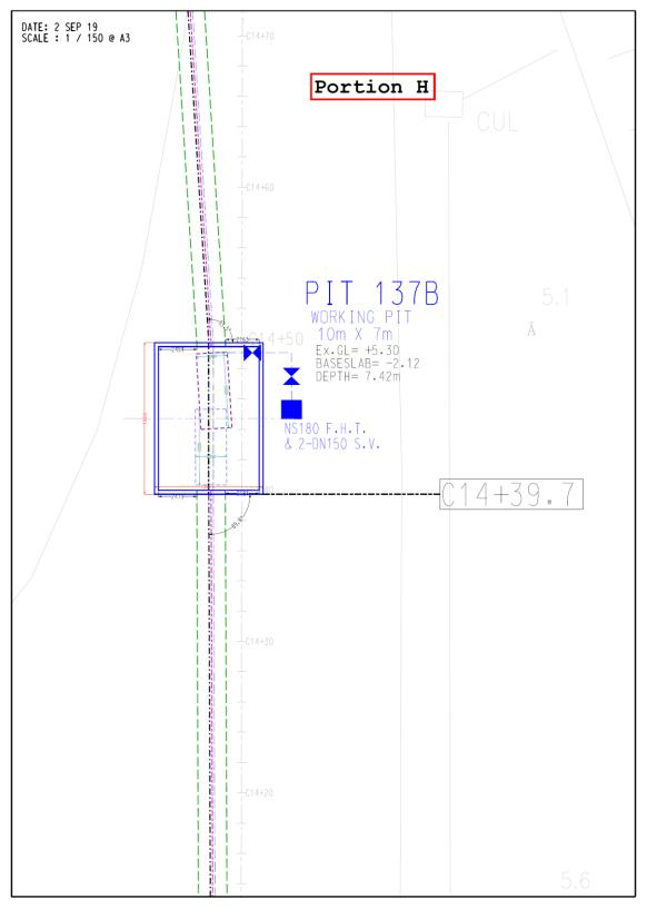
Figure B13a. Location Plan for Portion H– Pit 137B
