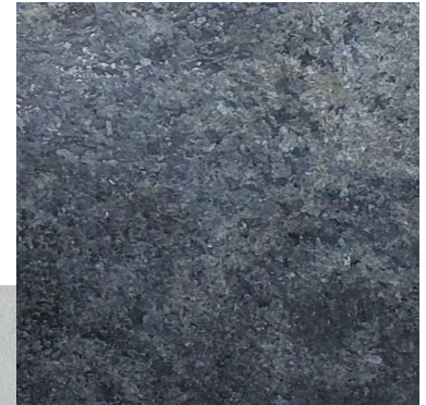
ST02 BLACK GRANITE WITH BUSH HAMMERED FINISH EDGE OF STEPS AT SAIRCASE AND PLANTER
