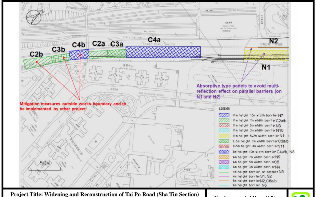
**Figure 2a: Locations of Noise Mitigation Measures (1 of 4)** (Extracted from Figure 2.1a of Environmental Permit Application No.: AEP-463/2013)
