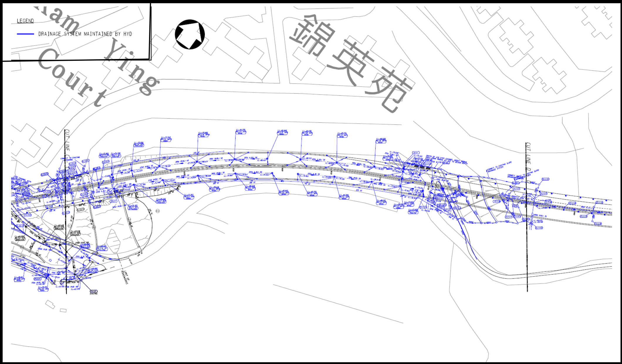
Project Title: Trunk Road T7 in Ma On Shan Figure H17: Drainage Plan of Highways Department (HYD) (Sheet 4 of 8)
